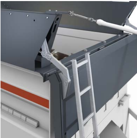
Ladder mounted at cutting table for easier service
